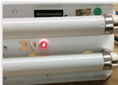
a. Power on L2 only(battery charging)
